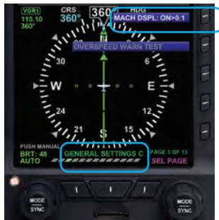
Figure 4-13b Speed Transition Setting
