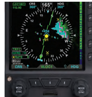
Figure 4-114 Navigation Display Showing Hazard Awareness
